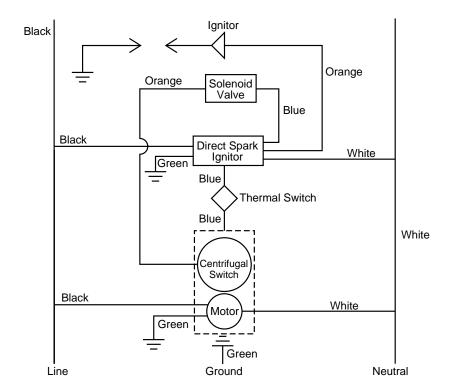
Figure 12 - Electrical Ladder Diagram
